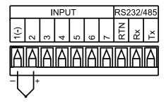
Figure 2.5 Thermocouple Wiring Hookup
